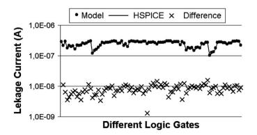
**Fig. 9.** Average leakage currents in 93 logic gates from GenLib\_44-6 library [17], using a 32 nm bulk CMOS PTM process [19].
