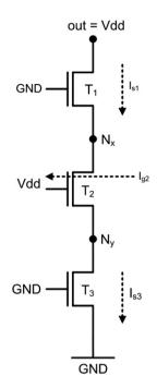
Fig. 2. Leakage currents in a three transistors stack.
