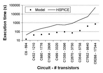
Fig. 12. Comparison of execution times.
