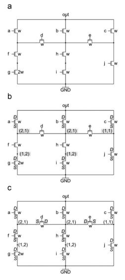
**Fig. 8.** Off-network representation: (a) originally extracted network; (b) assignments after steps 1, 2 and 3; (c) final transistor bias identification.
