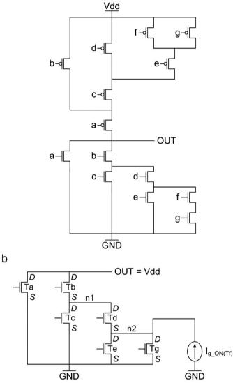
**Fig. 7.** Method illustration: (a) CMOS complex gates and (b) off-network representation for input vector [a, b, c, d, e, f, g]=[0,0,0,0,0,1,0].
