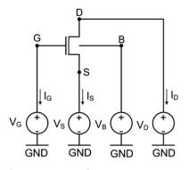
Fig. 5. Test structure for parameters extraction.
