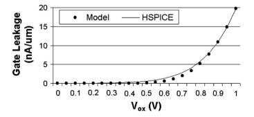
Fig. 4. Gate leakage current correlation of Eq. (5) to HSPICE data.
