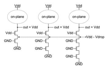
Fig. 11. On-devices on the top of stacks with different number of off-transistors.
