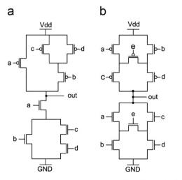
**Fig. 1.** CMOS complex gates: (a) out=!(a.(b+c.d)), and (b) out=!((a.(b+d.e))+(c.(d+b.e))).
