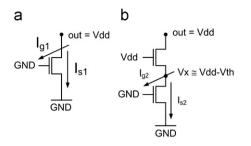
**Fig. 3.** Leakage currents in two different off-transistor conditions: (a) single offdevice and (b) two stacked transistors.
