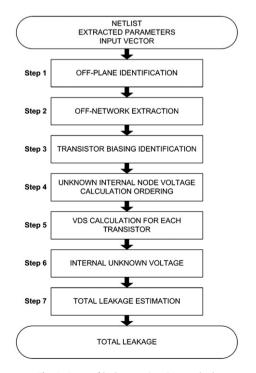
Fig. 6. Steps of leakage estimation method.
