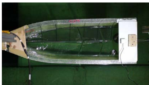
Fig. 2. A picture of the planing model with two swept steps from the top view.
