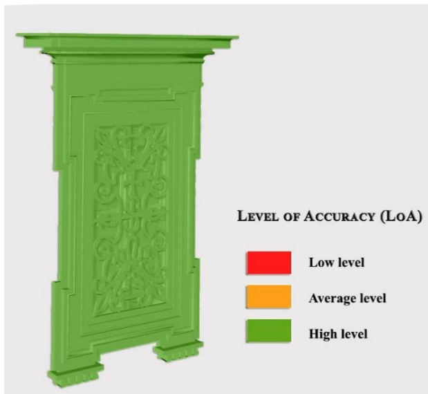
Figure 5: Level of Accuracy (LoA) of the model of St. Basilio's window: High LoA, that is 70% of the model has a deviation less than 20 mm, and 30% with a deviation less than 50 mm
