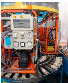
Fig. 3. Pump carousel used to perform vacuum creation in refrigerators (left); Pirani gauge used to assess vacuum quality (right).
