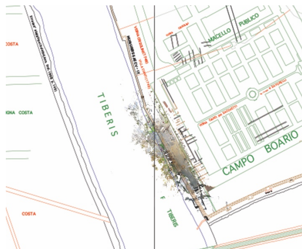
Figure 13. Overlap of the point cloud obtained by laser scanning, with the plan of the Forma Urbis of Rodolfo Lanciani
