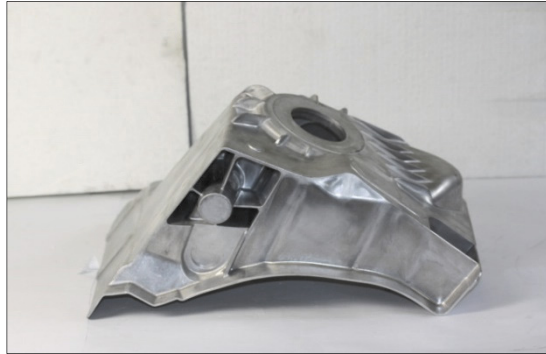
Fig. 1. Shock tower investigated in this work.
