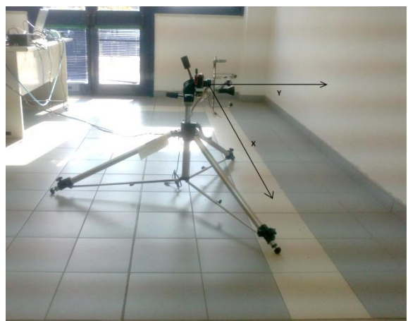
Figure 2. The scanning device for estimating the wall orientation
