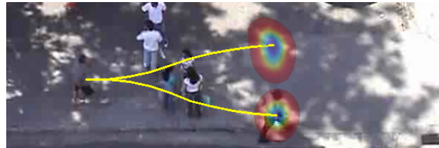
Figure 1. When moving through a scene, a person takes a variety of factors into account, such as steering clear of other people. In many cases, the prediction of the motion cannot be well described by a deterministic algorithm: in the above example the pedestrian on the left hand side could either evade the group by going on its left or right side, as indicated by the yellow lines. We therefore propose a stochastic, simulation-based motion model that can deal with the uncertain future motion of a pedestrian.
