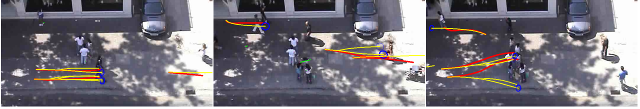
Figure 8. Typical failures of the sLTA: (Left, middle) unnecessary splittings can occur due to other wrong extrapolations, but are handled in the multi-hypothesis framework. (Right) without the knowledge of people walking in groups, wrong extrapolations can occur. (see text for details)
