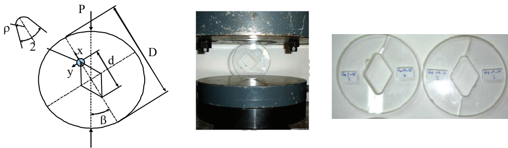
Figure 2: Geometry of the Brazilian disk weakened by blunt V-notches
