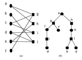
Fig. 1. (a) Example of Tanner graph containing a cycle of length 8  $\{d, l, e, h, a, g, c, i\}$ ; (b) A length  $\ell$  cycle can be found exploring the support tree up to level  $\ell/2$ : e.g., node d and  $\ell = 8$ .
