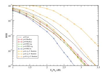
Fig. 2. BER as a function of SNR before and after girth conditioning for the MacKay's regular (504,252) code [22], the regular and irregular PEG (504,252), and the random regular ( $d_v = 5$ ) code. For comparison, BER of QC-LDPC(255, 510) after girth conditioning, as in [15], is reported.
