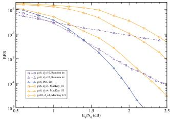
Fig. 4. BER as a function of SNR for some codes before and after girth conditioning: MacKay's regular (816,272) rate-1/3 code ( $d_v = 4$ ) [22] and irregular ( $d_v = 10$ ) random code. For comparison the performance of irregular PEG (1008,504) code is reported.
