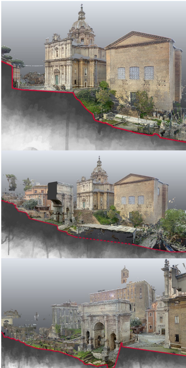
Figure 2: Perspective sections obtained by modifying the clipping box of ReCap. The particular orographic condition is highlighted by the complexity of the sections.
