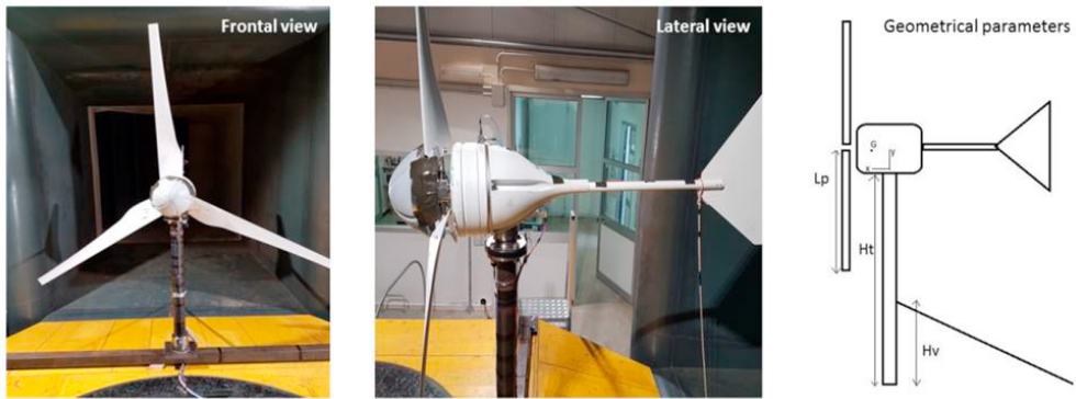
Fig. 3. Representation of the test case wind turbine and of its geometrical scheme
