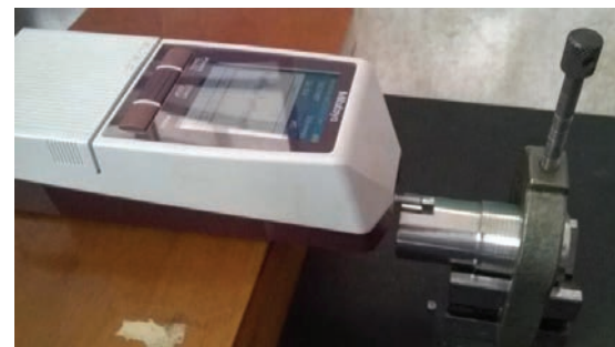
Fig. 3 Roughness measurement setup.
