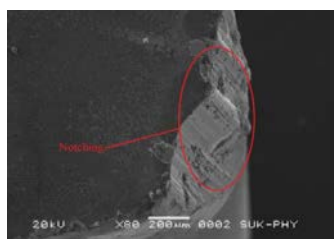
Fig. 9 Tool wear pattern at various speeds (SEM and HRP)
