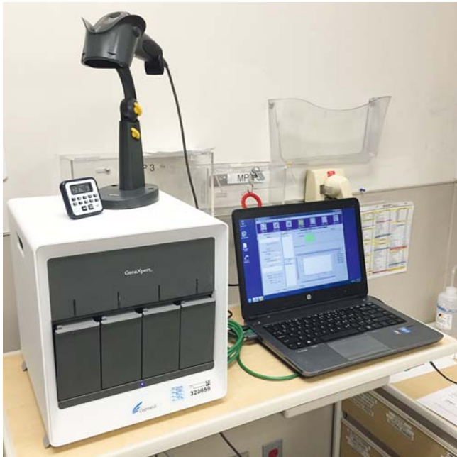
► Fig. 1 Four-module Xpert instrument that runs the CARBA-R CRO (Cepheid, Sunnyvale, California, United States) assay with associated laptop computer in the preoperative area of the endoscopy suite.
