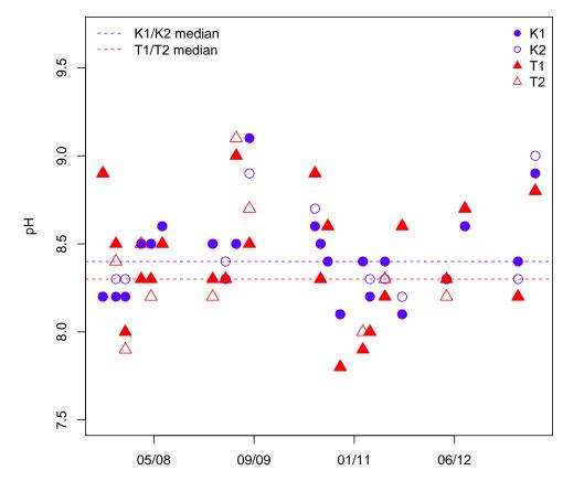
Figure 7: The pH levels were measured in the laboratory using surface water samples collected at 0.3 m. The median pH values at all sites were very similar (K1/K2 = 8.4; T1/T2 = 8.3). All pH levels were slightly alkaline (>7), and most were >8.0, which is typical for lakes with high conductivities and high algal concentrations (Figure 14, page 17)
