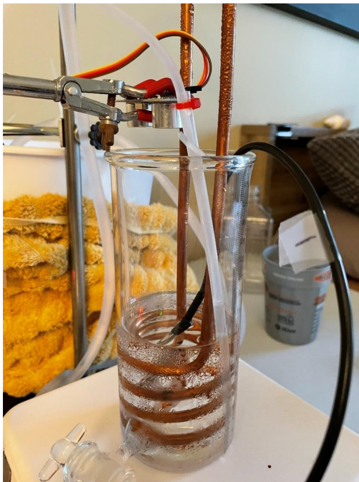
Figure 7: Reaction vessel and exchanger with internal temperature probe and HC-SR04 ultrasonic sensor.
