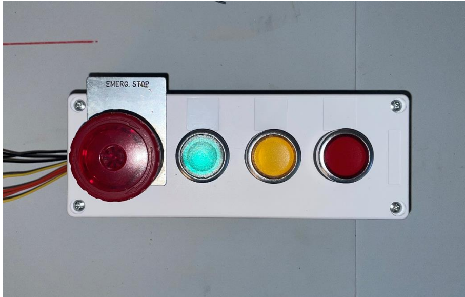
Figure 4: Four button panel fabricated for control system. Left to right: RED – Emergency Stop, GRN – Start, YEL – User-Programmable, RED – Normal Stop.
