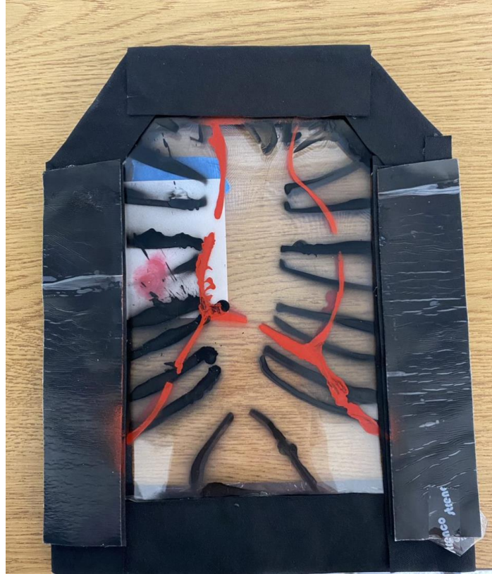
Post .357 Magnum Test (No Trauma Pad) – Impact Is Very Visible on Sample (Left Side of Clear Vinyl)
