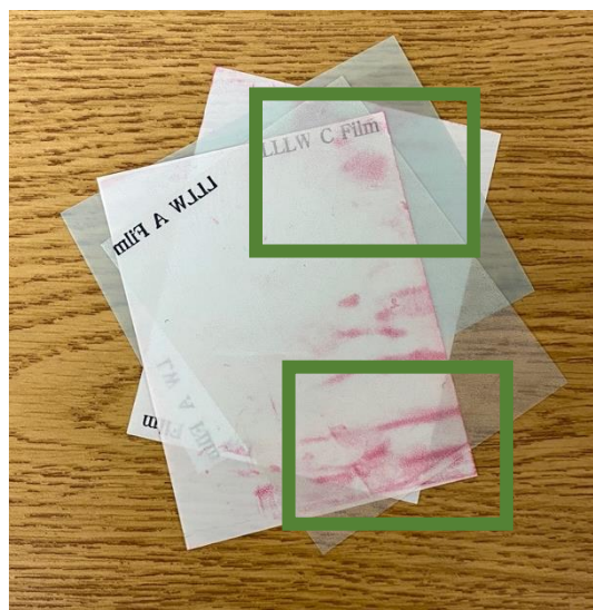
9mm Film Samples After Initial Tests
