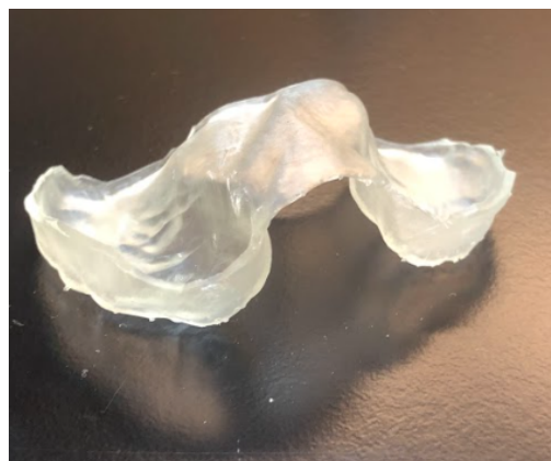
Figure 3: First 3D printed NAM aligner that was printed for validation testing.
