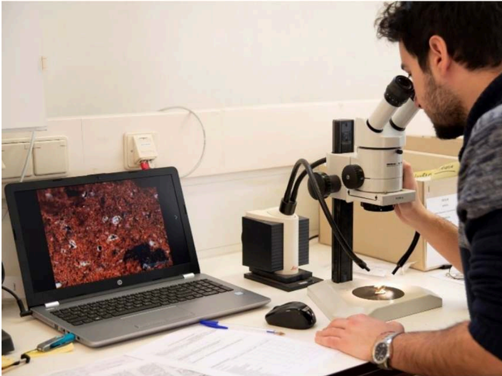
Fig. 2. Autoptical analysis of the fabrics with the optical microscope. University of Vienna, 2018/2019
