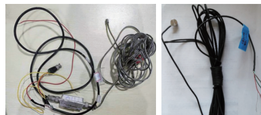
(a) Pore water pressure transducer (b) Soil stress transducer
