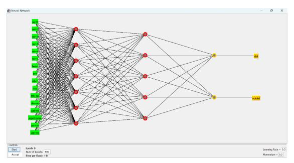
**Figure 5.** Structure of MLP architecture using the dataset attributes (su, hemo, pcv, wbcc, rbcc, htn, dm, cad, appet, pe and ane) in two hidden layers. The Feed-forward neural network connecting all the neurons appears to be less intricately connected to the dataset attributes chosen.
