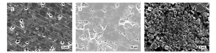
SEM micrographs of BTO sintered under different conditions: (a) flash sintering of micropowder (~2 μm) at 150 V/cm and 15 mA/mm<sup>2</sup>; (b) conventionally sintering of nanopowder (~100 nm) at 1400 °C for 4 hours; (c) flash sintering of nanopowder at 150 V/cm and 15 mA/mm<sup>2</sup>. Different microstructures are obtained deppending on the green powder and sintering approach.
