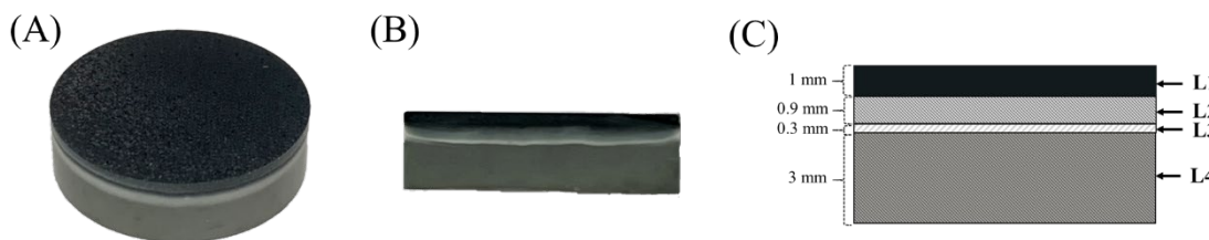
Figure 1 – Images of the bi-layer DHGI sintered by SPS; A) Top view, B) Side view and C) schematic illustration.
