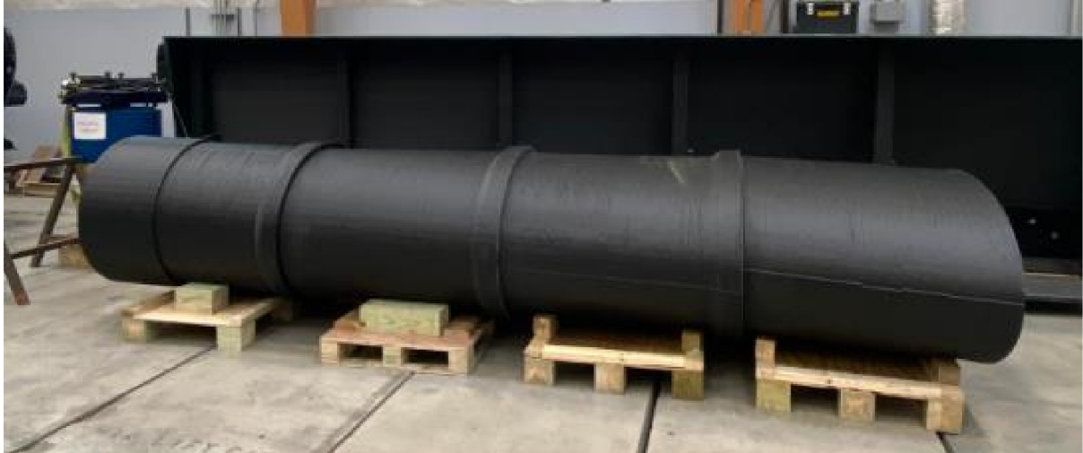
Figure 8.2: Assembled large-scale 3D printed highway culvert diffuser.
