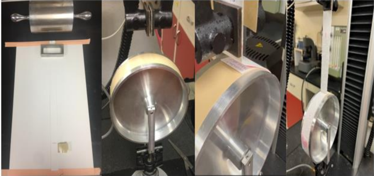
Figure 6.6. From left to right respectively: spreading adhesive onto one strip of paper flat on the table using block coater and pressing using a roll; double side tape fixed to the peel wheel clamped in the Instron; glued sample fixed to the peel wheel; and sample being peeled few minutes after starting peeling test.
