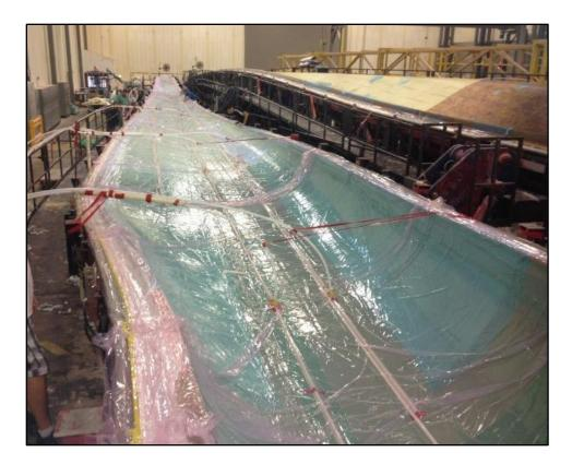
Figure 3: Large-scale Vacuum Infusion (Provided by TPI Composites Inc.) [10]
