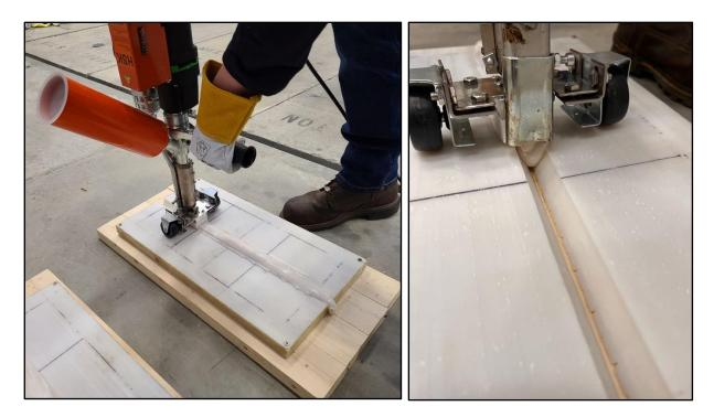
Figure 22: Extrusion Welding AM Plate
