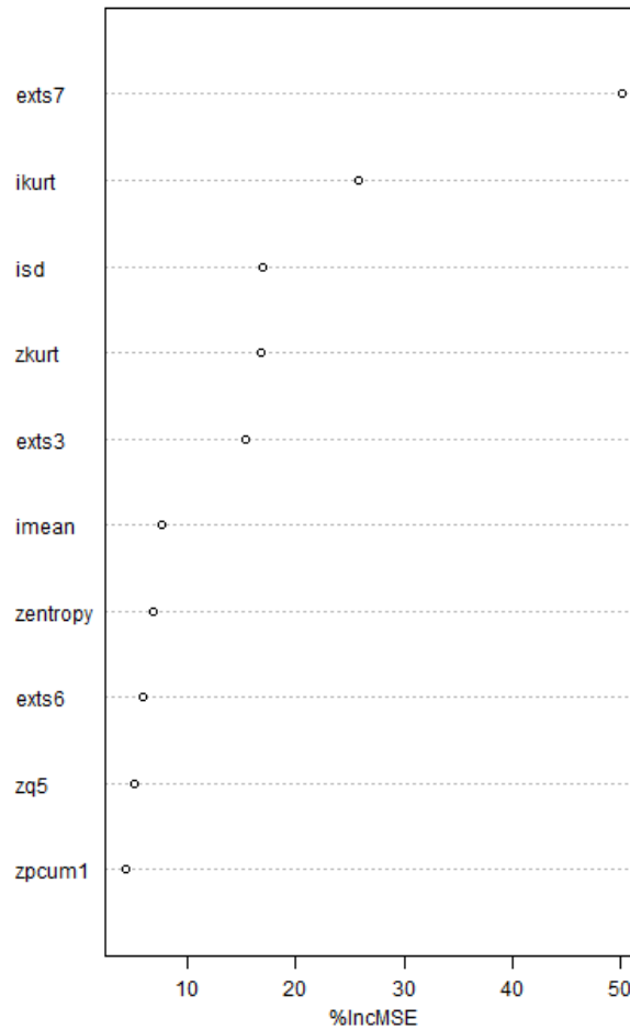
Figure 2.3. The ten most important percent softwood predictor variables for the PEF model using 92 FRPs and a PCA for plot placement.
