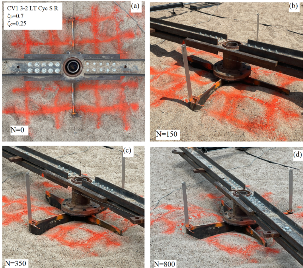
Figure 5.15: Soil subsidence around the CV1 3-2 after N cycles in the sand.
