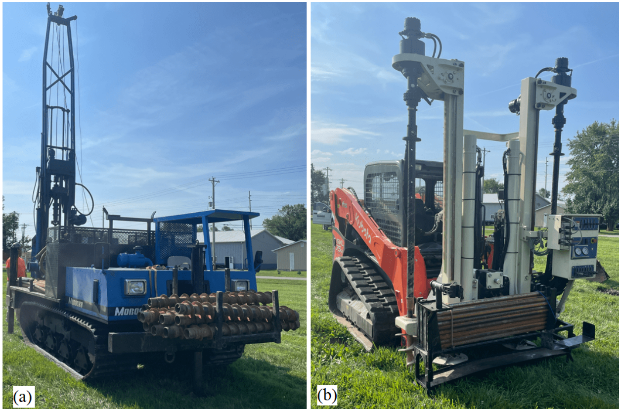
Figure 3.7: (a) CME-55 Truck Mounted Drill and; (b) Kubota SVL 75-2 equipped with a Geoprobe 20CPT.
