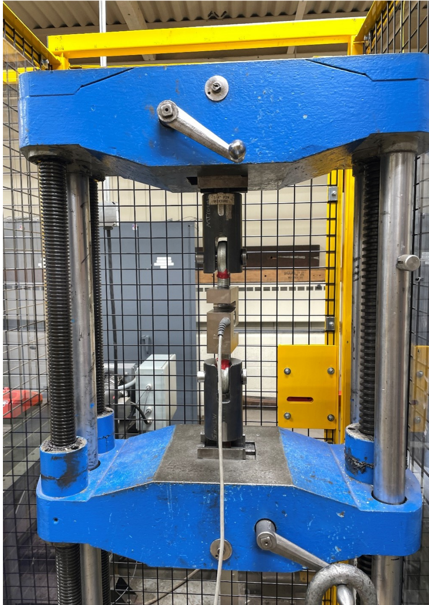
Figure A.3: STA-4 S-Type Load Cell Calibration in test frame.
