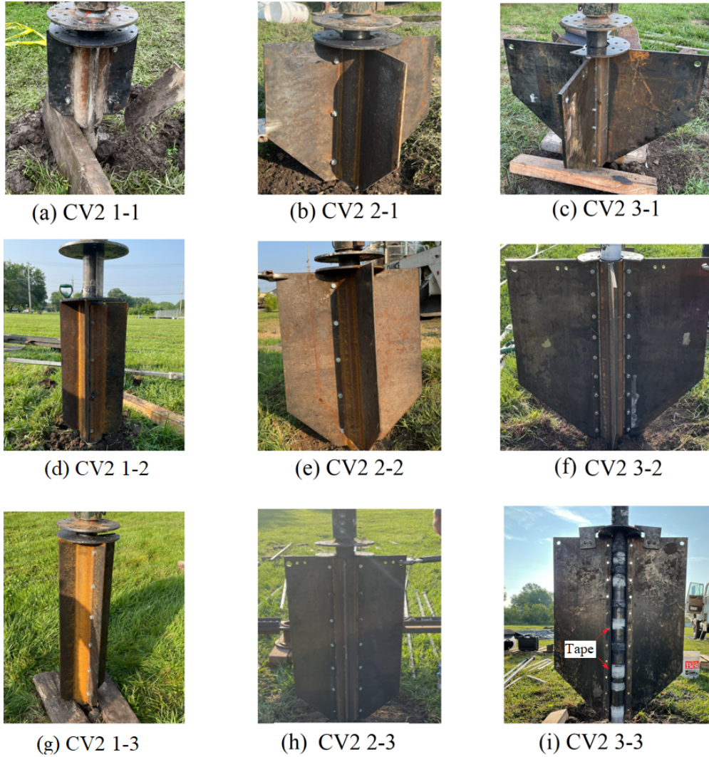
Figure 3.1: Two-piece Collar Vane (CV2) geometries.
