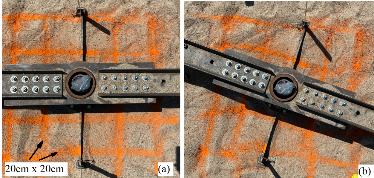
Figure 4.22: CV1 3-2 LT S under torsional loads in the sand.
