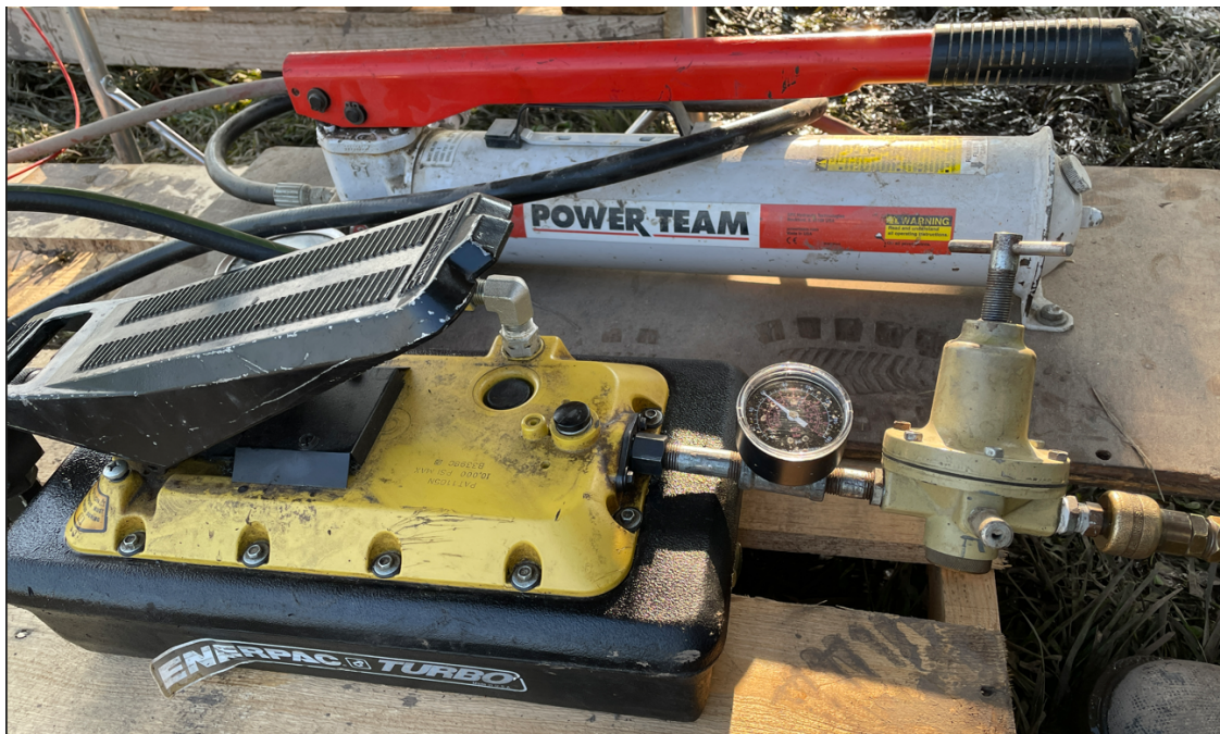
Figure 3.12: Enerpac PAT1105N foot pump (front) and Power Team P159 hand pump (back).
