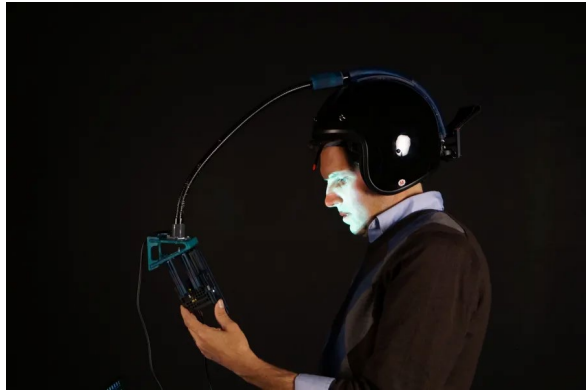
Siavash Tohidi (In collaboration with Dr. Daniel Lau and Dr. Michael Winkler)*, Digital Skin/Face Paint , 2019-20, Intel RealSense SR300 Camera and projector mounted on motorbike helmet with custom-build attachment, 3-D resin-printed housing, and 3-D filament-printed parts
