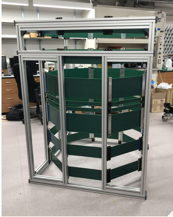
Figure 3.15: Picture of the half-scale prototype B_0 coil.
