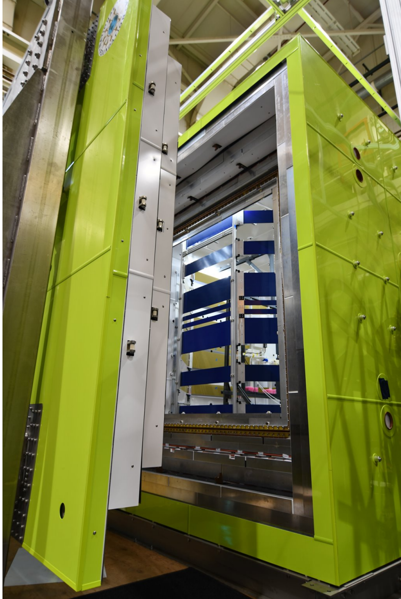
Figure 3.14: Picture of the full-scale B_0 coil assembled in the MSR at LANL.
