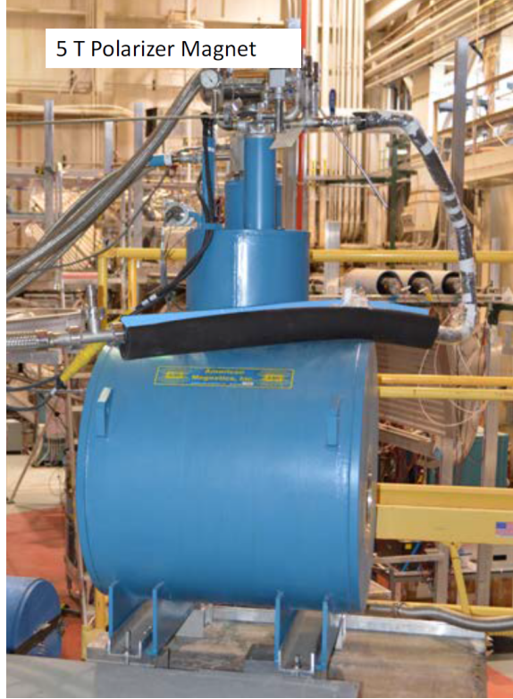
Figure 2.6: Picture of the 5 T superconducting solenoidal polarizing magnet to be used in the LANL-nEDM experiment. [41]
