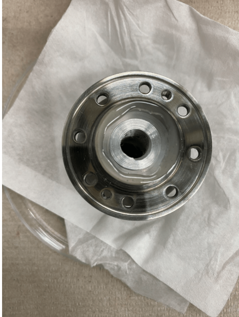
Figure 2: Epoxy application on the window.
