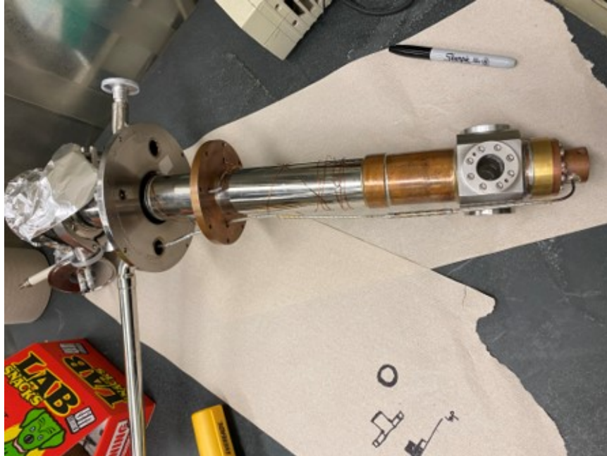
Figure 1: Inner vacuum system.
