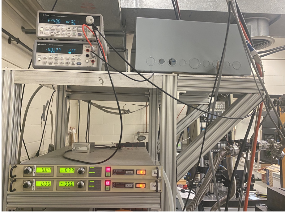
Figure 6.4: At the bottom left of the picture are two Spellman SL30PN150 high voltage (HV) power sources. The top items on the top shelf are a waveform generator and a digital multimeter.
