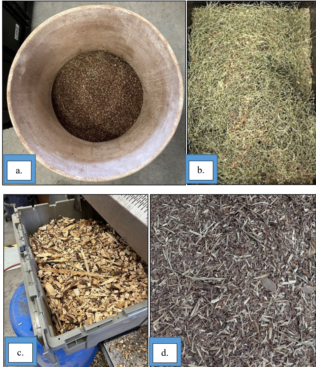
Figure 18. Air classified fractions including a) fines/dirt rich, b) needle rich, c) white wood rich, and d) bark rich.
