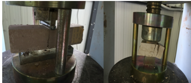
Figure 2 Flexural and compressive strength tests
