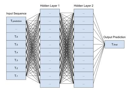
Figure 2.1: Depicting the dense nature of the hidden layers, each layer has output to every layer in the next hidden layer.
