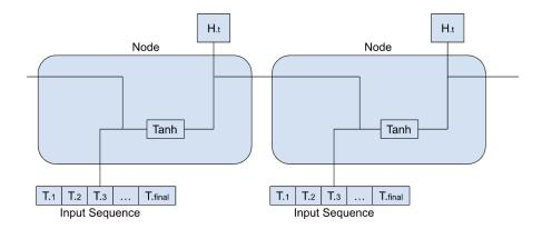
Figure 2.2: Depicting how each node of the LSTM model has a forget gate in addition to its input and outputs.
