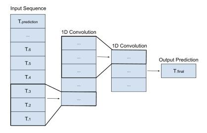
Figure 2.3: Depicts how each window of the CNN model is able to learn from not only the inputs surrounding it but also the surrounding convolutional layers.
