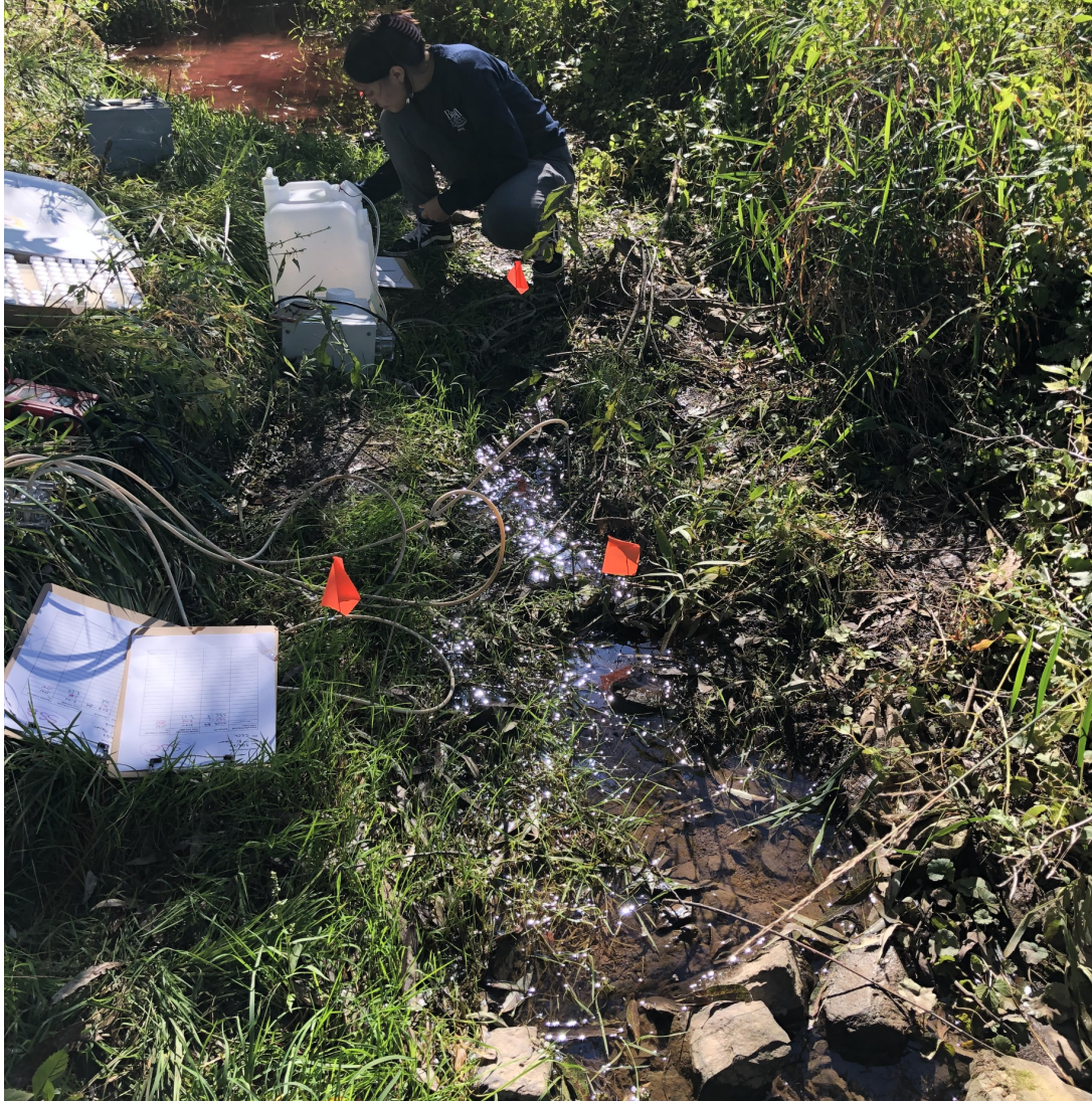
Figure 38.) Tracer setup, sampling locations marked by flags, and some transient storage zones.
