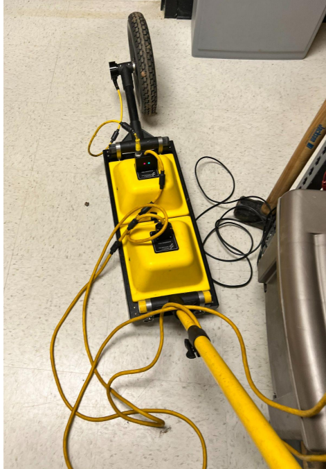
Figure 9.) GPR setup using a trolley to hold the transceiver and receiver. Photo courtesy of Rob Jacob.
