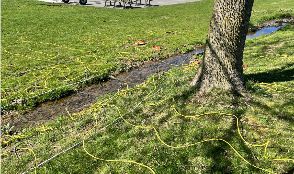
Figure 8.) Basic setup that shows correct spacing. Yellow cables are the electrode lines that are resting on contact probes.
