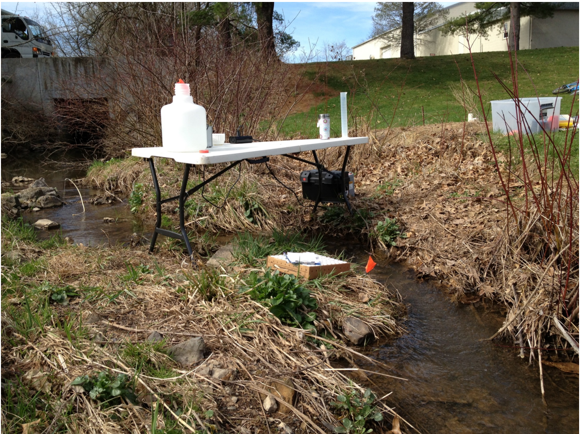
Figure 10.) Example tracer injection and sampling site. Injection happened at the white table and samples were collected downstream at the orange flag and at additional locations not shown in the image.
