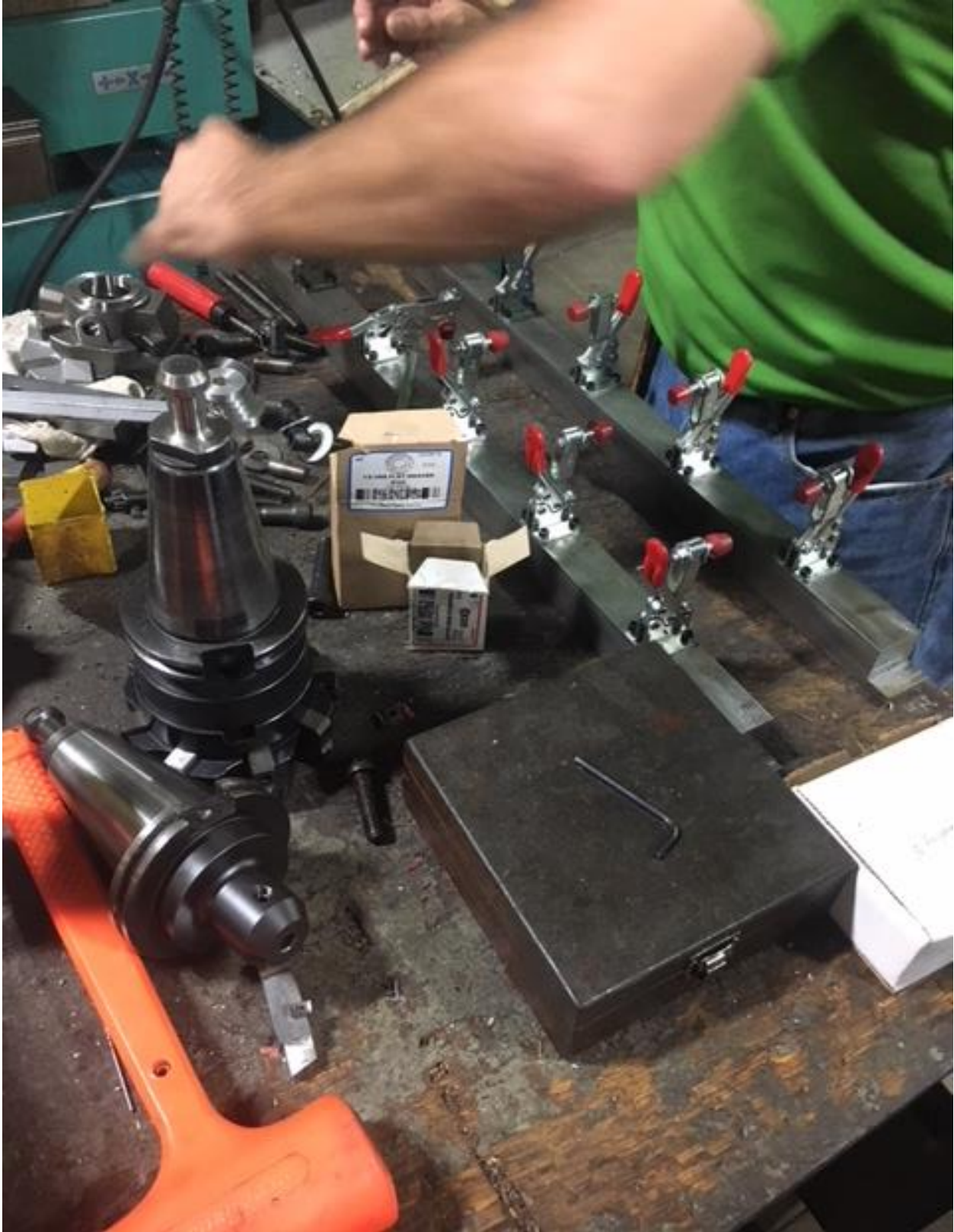
Figure 24: Machinist Denis of MAGSEAL illustrates the current clamp mechanism with a series of rubber stops, which is an arduous process to set up.
