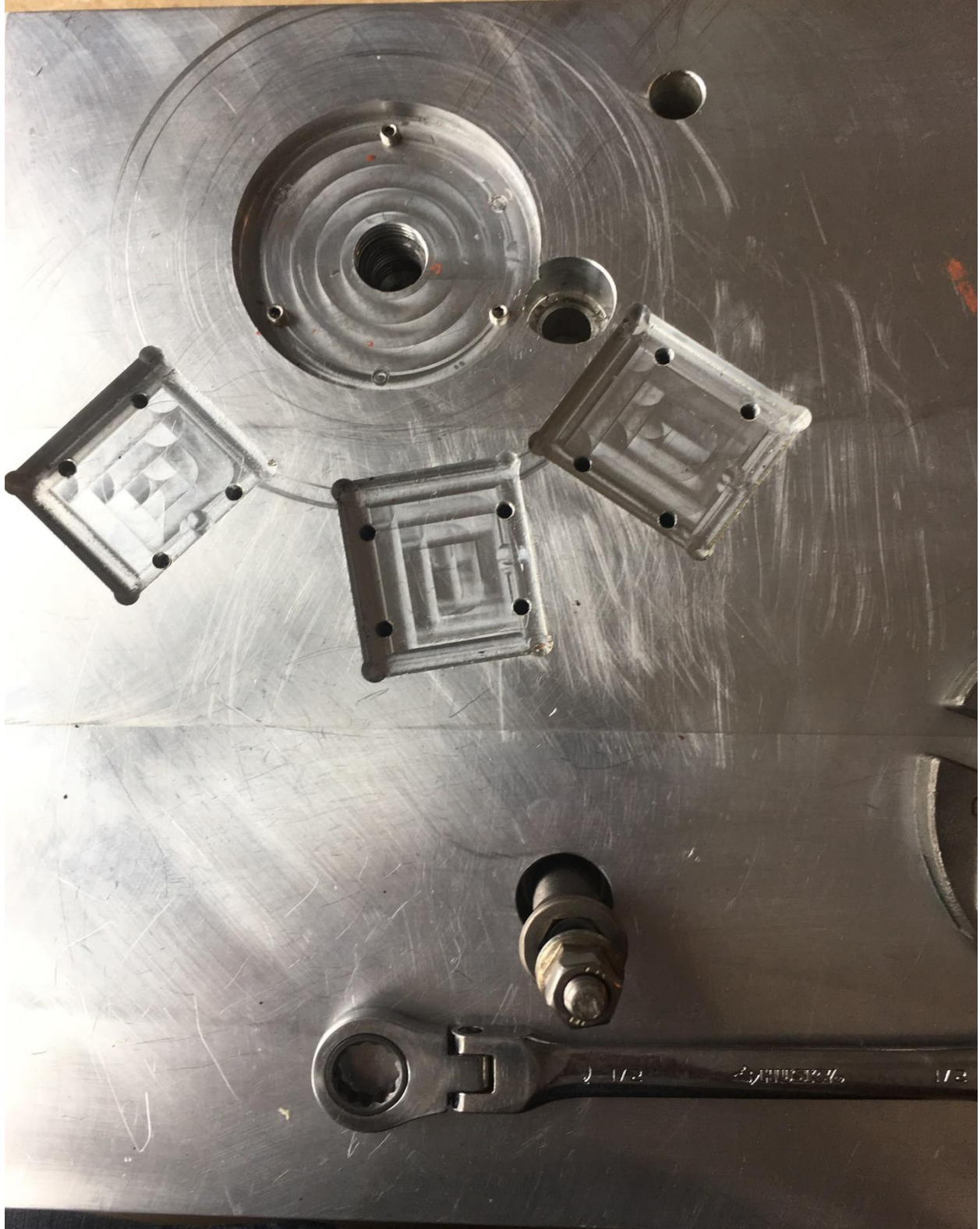
Figure 27: The aluminum base plate has a counterbore for the collets to be easily interchanged. It also has rectangular extrusions for the slide-lock mechanisms depending on the angle needed for drilling. Unlike the previous design, both the clamping and orienting features are all comprised in one unit.
