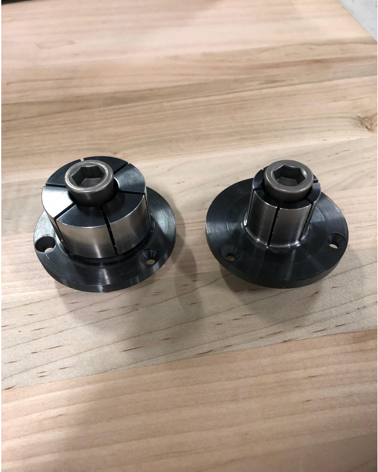
Figure 26: The modified Mitee Bite ID Expansion collets turned down to for the larger sized gland seal (left) and the smaller sized gland seal (right). The flange diameter for both pieces is the same and allows for quick changeability and less custom parts.
