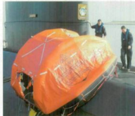
Blow-up: The self-inflating raft, which contains GPS and supplies, can be deployed inside the pressure hull or topside
