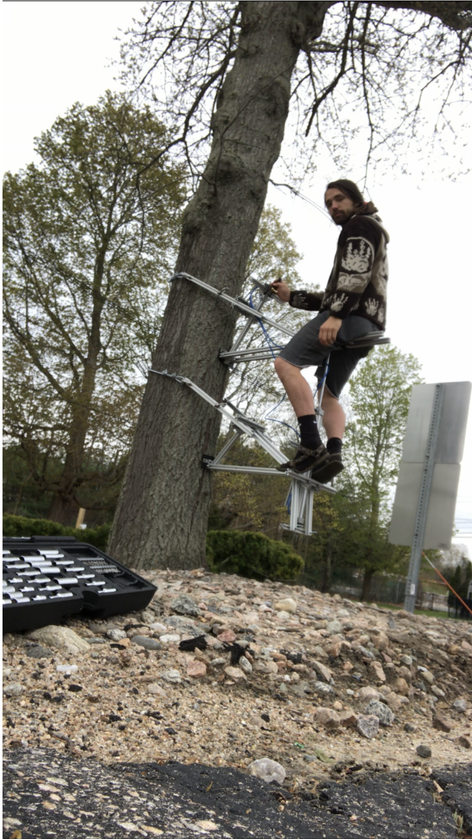
Figure 30: Pneumatic Stepper (Final Design, weighted my Scott Botelho)
