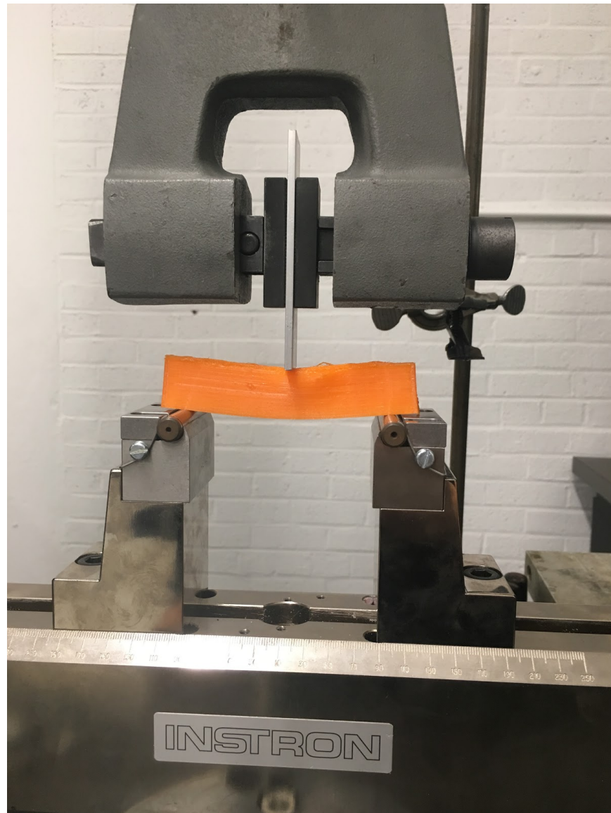
Figure (30): Image of Honeycomb in 3-point bending
