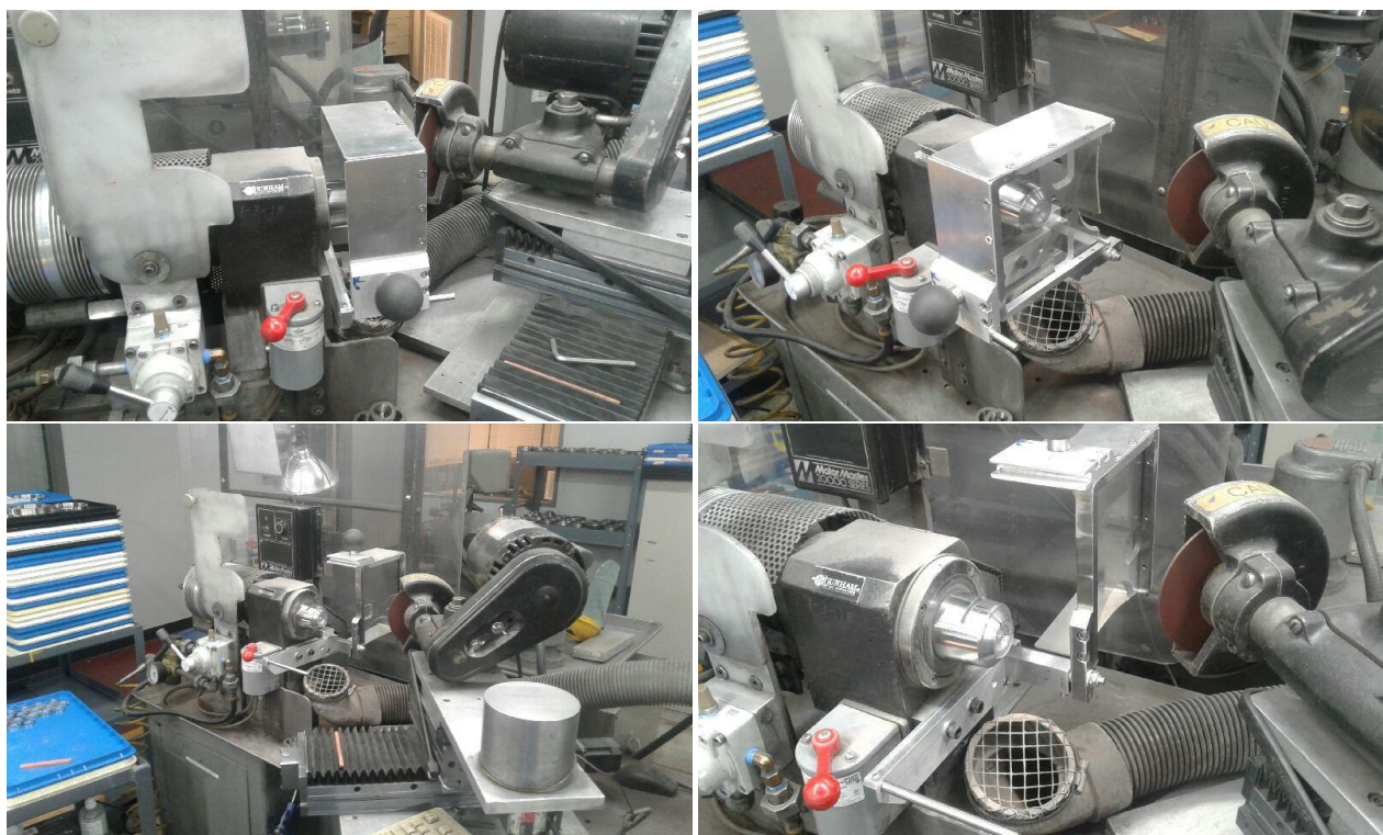
Figure 60: Guard Mounted to Deburring and Chamfering Machine
