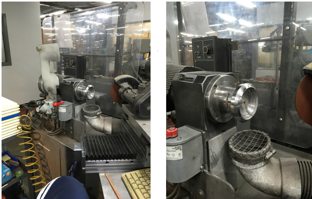
Figure 3: Deburring and Chamfering Machine at its Current State
