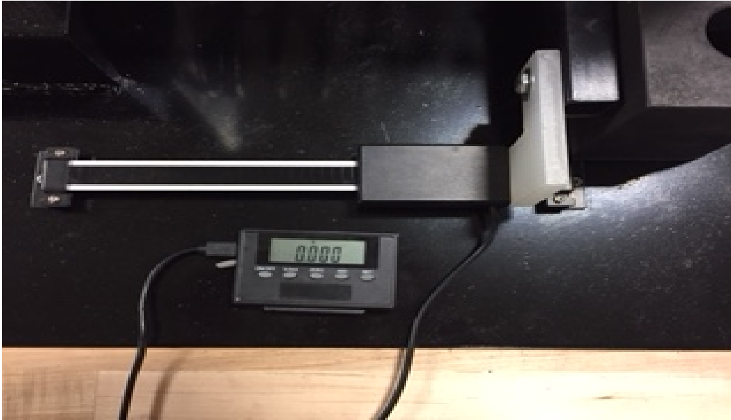
Figure 136: Turn on DRO and zero
