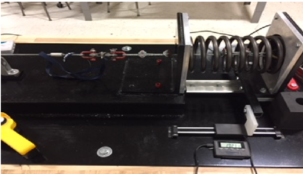
Figure 139: Pull spring to desired displacement shown on DRO
