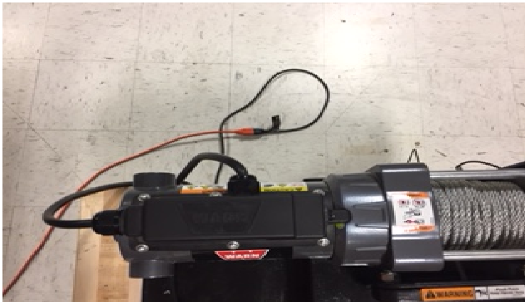
Figure 135: Connect winch to power supply
