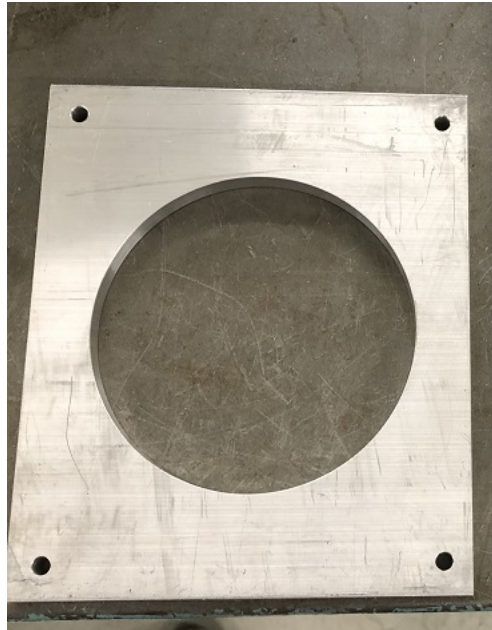
Figure 130: CNC Milled Aluminum Spring Housing
