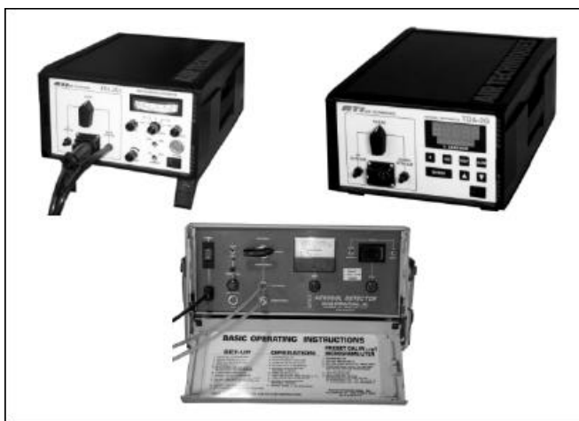
Figure 8.6 – Commercially Available Packaged Forward-light Scattering Photometer for HEPA Filter In-place Testing
