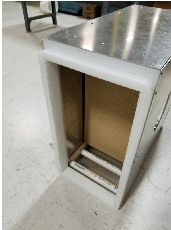
Figure 24: Test Build Bagging Ring and Rollers
