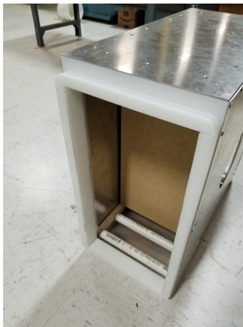
Figure 17: HEPA Filter Housing Test Build
