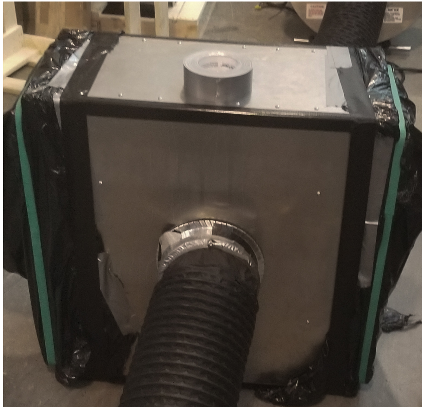
Figure 21: Test Housing Inlet
