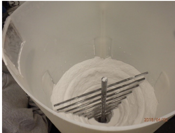
Figure 58: Flow Stagnation during Testing
