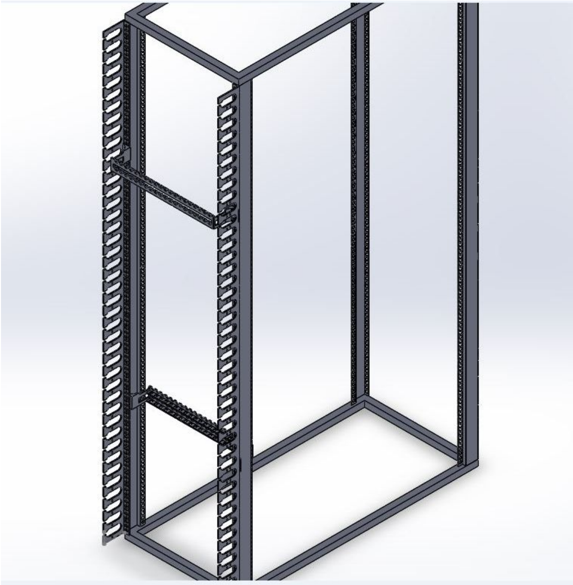
Figure 54: Assembly of cable management pieces on rack
