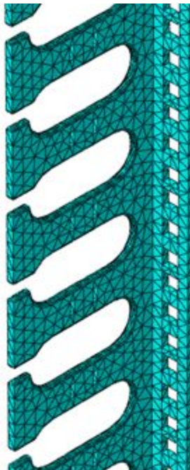
Figure 51: Abaqus mesh of vertical component
