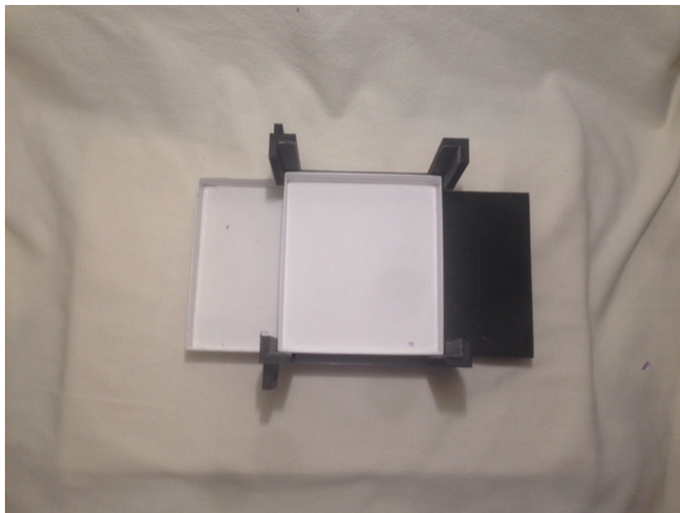
Figure 33: Box bottom loader half way through dispensing cycle
