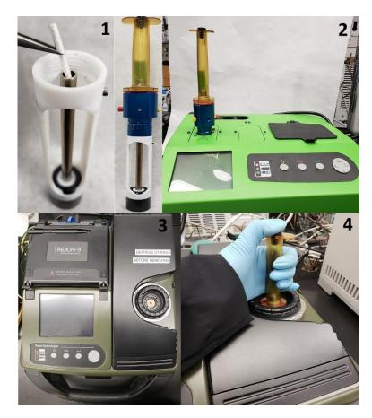
Figure 17: Picture scheme of the CMV/NTD sampling protocol. CMV is inserted into the stainless-steel tube and sealed with the NT adapter (1). Holder with inserted needle trap is placed into SPS-3 for desorption method (2). Top view of the T9 portable GC-MS (3). Injection of the needle trap into the T9 after CMV desorption (4)
