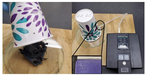
Figure 22: Photograph depiction of the CMV/Cup apparatus with debris placed on the glass platform (left) and the CMV sampling using the hand-held vacuum pump (right)
