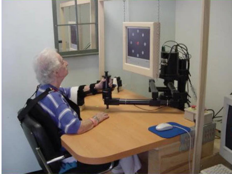
Figure 1.2: MANUS device. Pictured is the SCARA arm holding the force sensor in the handle, with the visual feedback screen located above the table. Image credit [18]
