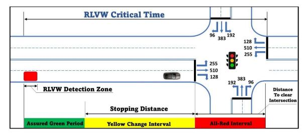
Figure 3-1: Case Study Signalized Intersection for Modeling RLVW Application
