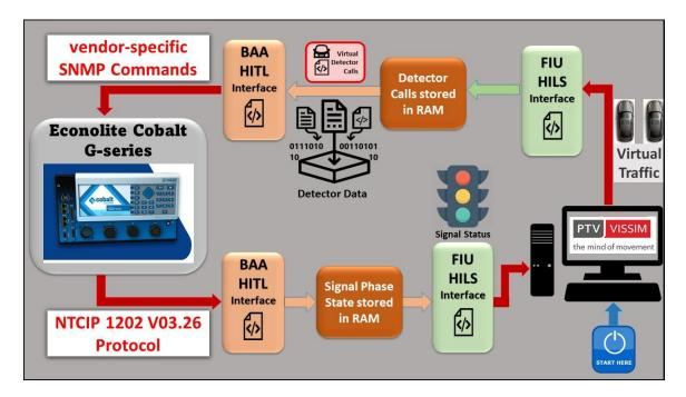
**Figure 3-3: Data Flow between the HILS Hardware and Software Components**
