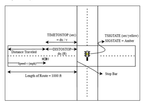
Figure 3-7: Variables Affecting the Stop Decisions in the Simulation Model
