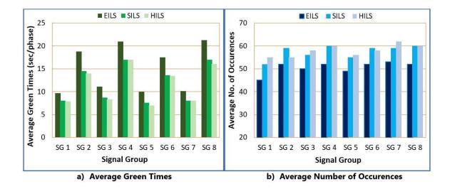
**Figure 4-2: Signal timing MOEs results**
