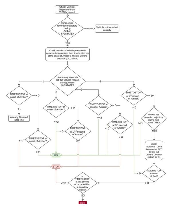
Figure 3-8: Vehicle Trajectories Analysis
