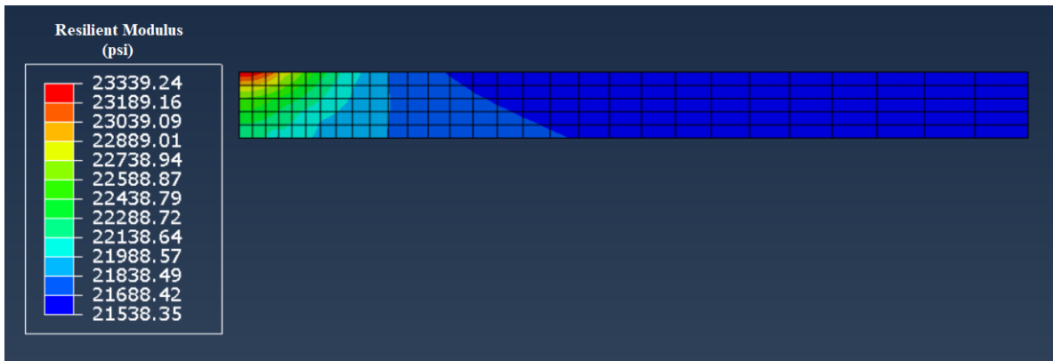
Figure 23: Contour of Predicted Resilient Modulus by ABAQUS Software for the Base Layer
