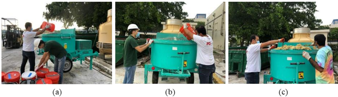
Figure 4.18: Sequence of adding material, (a) adding dry constituents and mix for 10 minutes, (b) adding water and chemical admixtures, and (c) adding fibers
