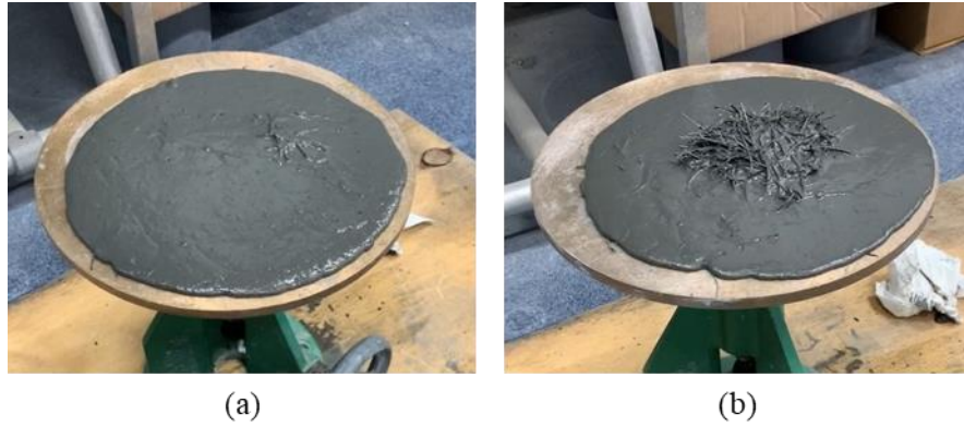
Figure 4.4: Photographs of two flow table tests performed on C6 with poor fiber distribution, (a) without many fibers and (b) with all fibers clumped in middle of test
